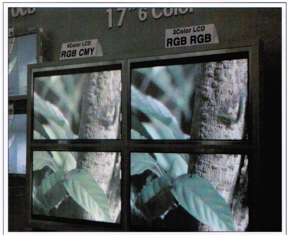
Fig. 4: Samsung's 17-in. WXGA display with pixels containing six different colored subpixels provided more-subtle color renditions and an expanded color gamut.
