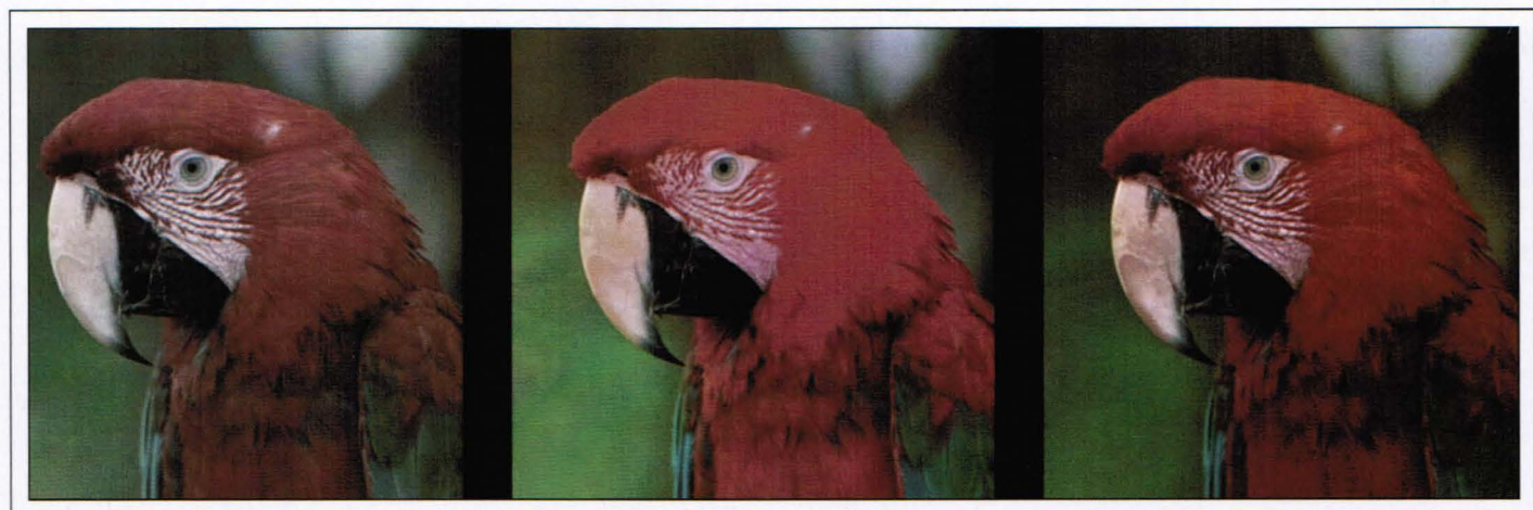
Fig. 3: The photograph on the left shows a typical mobile-display image without color processing; the image looks rather pale. By simple color processing, the photograph in the center shows improved colorfulness, but with visible clipping artifacts. Advanced color-gamut mapping shown on the photograph on the right preserves the colorfulness while eliminating clipping artifacts.
