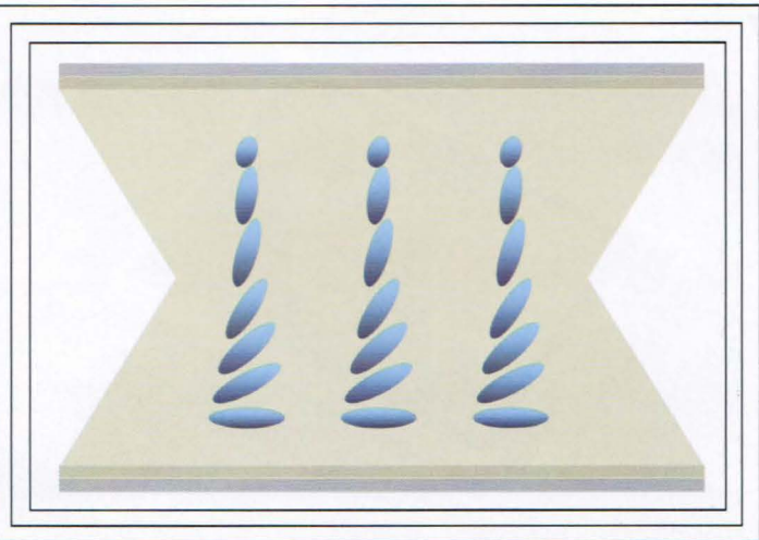
Fig. 2: The typical arrangement of a twisted-nematic liquid-crystal cell in the ON (light-conducting) state is shown. Light is polarized in fewer directions by the liquid crystals, resulting in a much narrower viewing angle.
