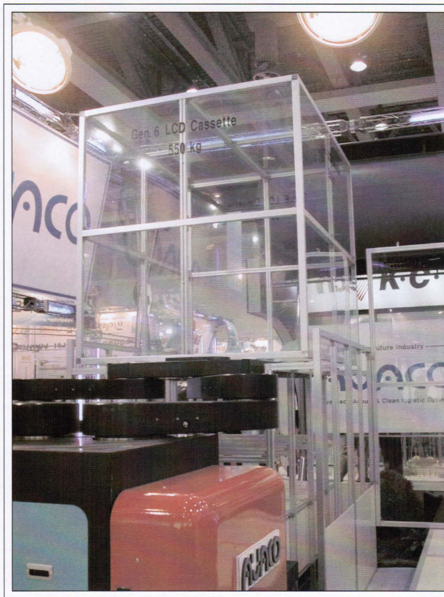
Fig. 5: AVACO's cassette-transfer robot system can lift and position loaded Gen 6 cassettes weighing 550 kg.
